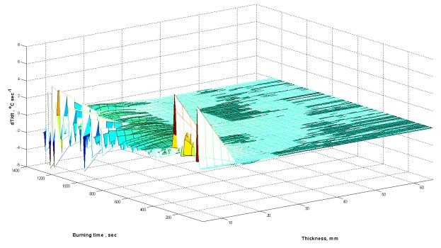
Fig. 7. Velocity of temperature change in spruce wood depending on the burning time and depths of the material
