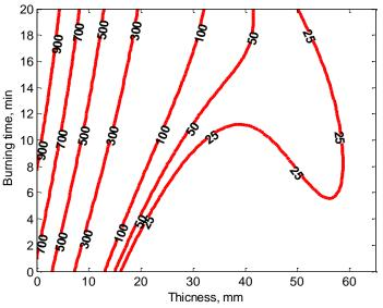
Fig. 5. Contour plot of temperature distribution in the spruce sample
