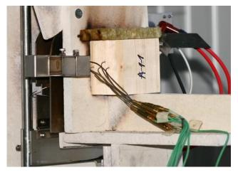
Fig. 1. Measuring the temperature of a wood sample during combustion
