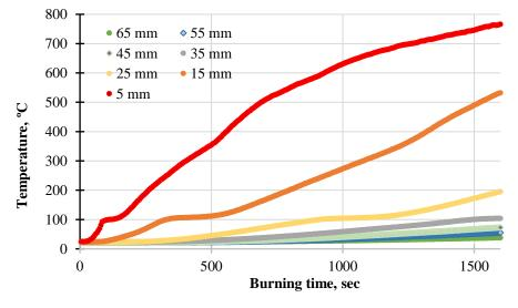
Fig. 3. Dependence of the temperature change on the burning time in different depths of spruce wood
